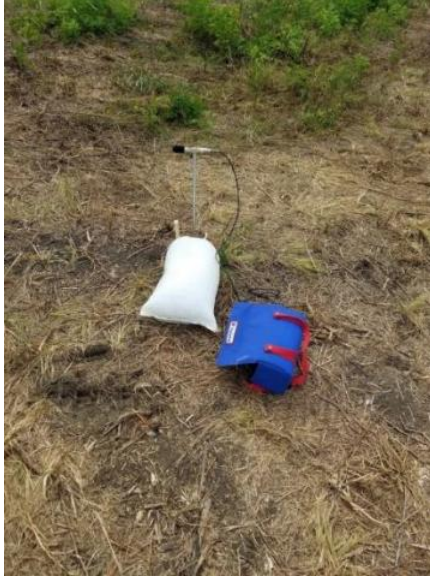
Figure A.16. Photographs of the instantel minimate blast seismographs installed before blast-induced liquefaction tests (Photo courtesy by the author).
