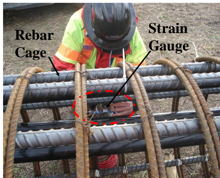
Figure A.10. Photograph of the linear vibrating wire strain gauge being mounted on the reinforcement cage (Photo courtesy of Sarah Bey, Bey 2014).
