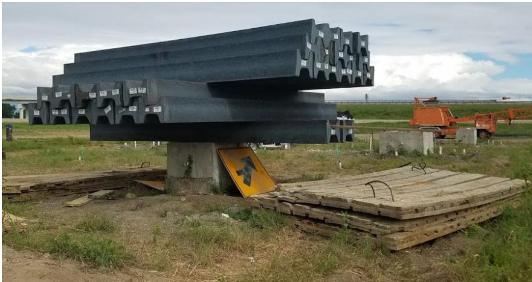
Figure 3.2. A photograph of a dead weight being applied to a drilled shaft foundation (photo courtesy of Elvis Ishimwe).
