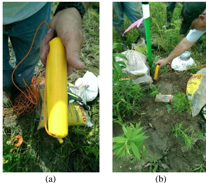
Figure A.19. Photographs of (a) the Dyno emulsion explosive, and (b) the charge being placed into the pre-drilled and cased hole (Photo courtesy by the author).
